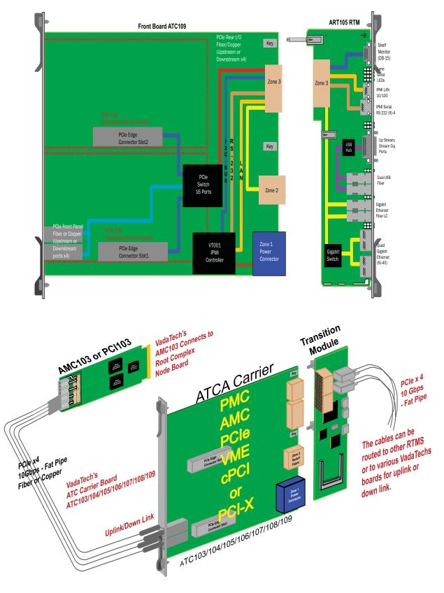
FIGURE 1. ATC109 Functional Block Diagram and a typical application (the module could run standalone)
